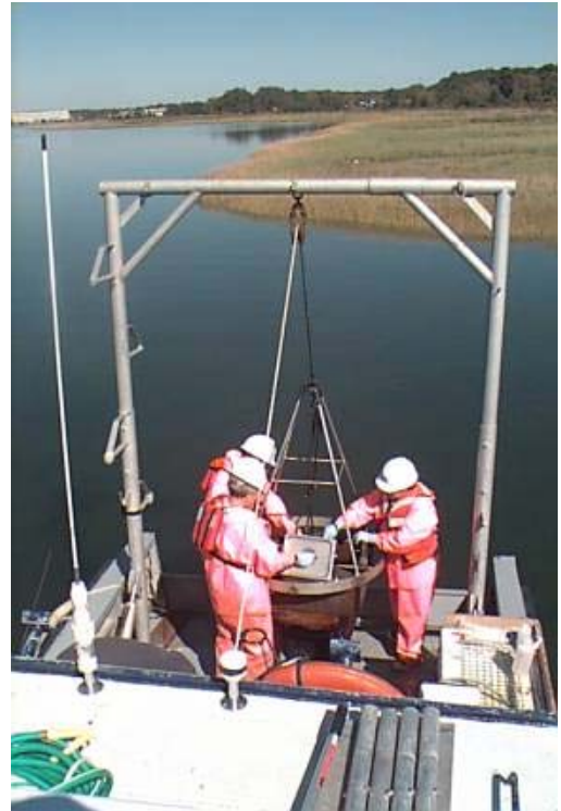
Sediment sampling and sieving on the deck of the R/V Cyprinodon.
