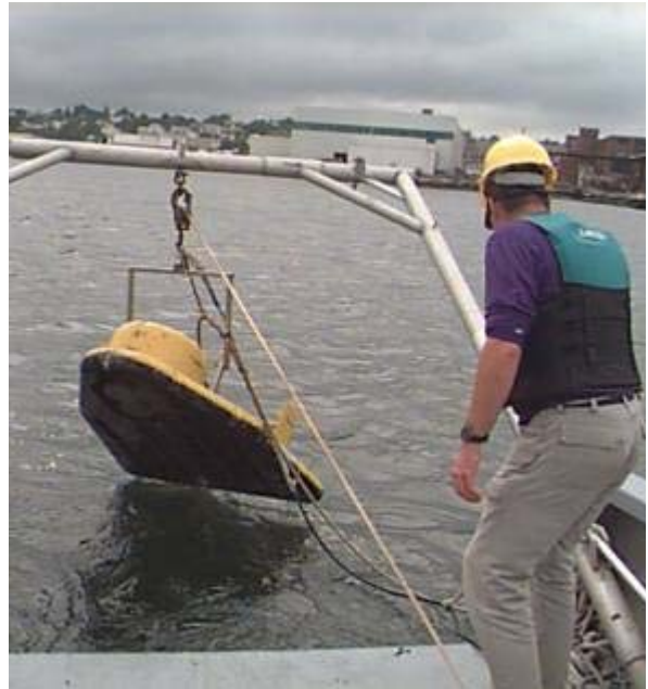
Deploying the sub-bottom towfish aboard the R/V Cyprinodon.
