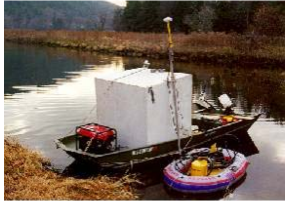
Shallow water survey jon-boat with a Honda generator, Trimble GPS, echosounder, and HYPACK survey software. The X-Star sub-bottom profiler was towed in an inflatable boat.
