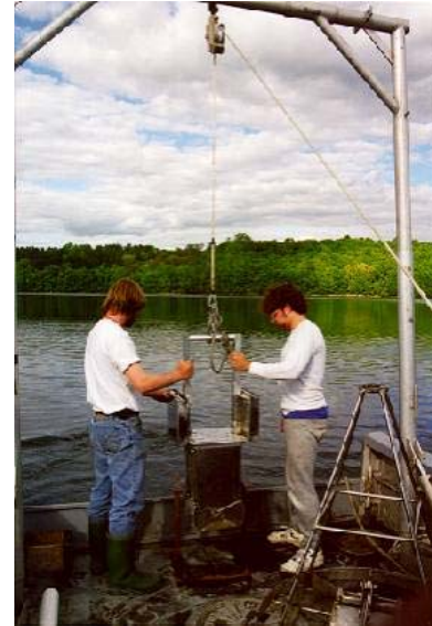
Box coring operation in Rondout Reservoir off the stern of R/V Cyprinodon.
