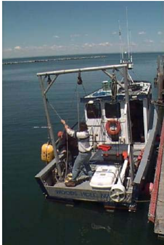
R/V Cyprinodon outfitted with Geometrics magnetometer, Klein side-scan sonar, and ORE sub-bottom profiler for the Long Island cable survey.
