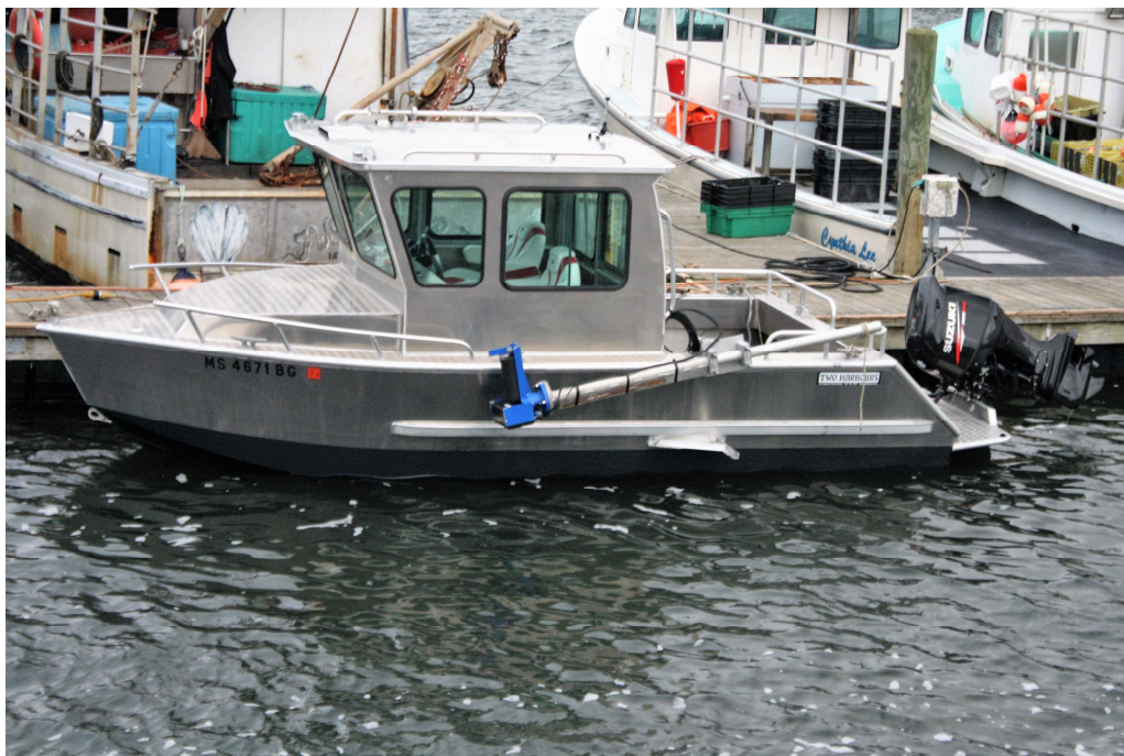
25-foot Bayview aluminum survey boat designed for inshore multibeam bathymetric and geophysical surveys
